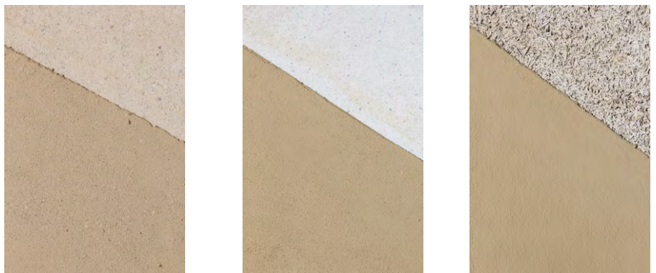
Examples of Léém Clay Plaster on suitable substrates: Léém Compressed Block, hempcrete block and gypsum fibre board (Fermacell)
