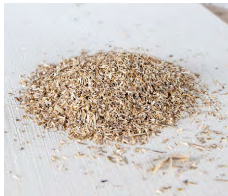
Straw fibres as a potential addition to the Léém Clay Plaster and finish
