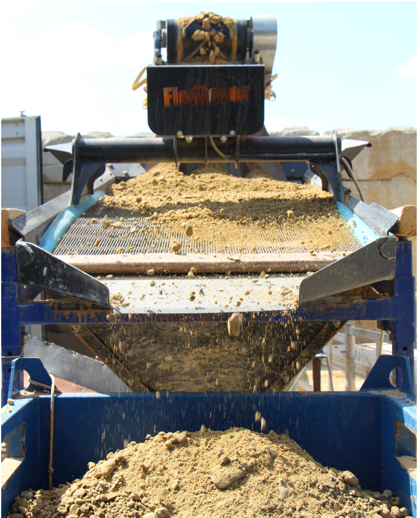
Sieving the local earth to valorise a 'waste' stream
