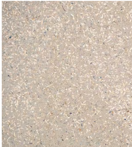
Léém Clay Plaster with a high quantity of additional straw fibres
